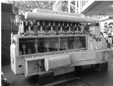
Figure: Power unit (engine and generator right) from a diesel-electric locomotive
